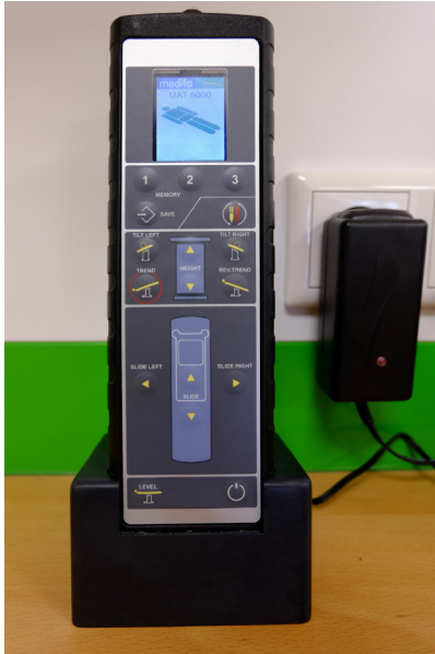
Fig. 21: Charging station with mains plug for the infrared manual switch
