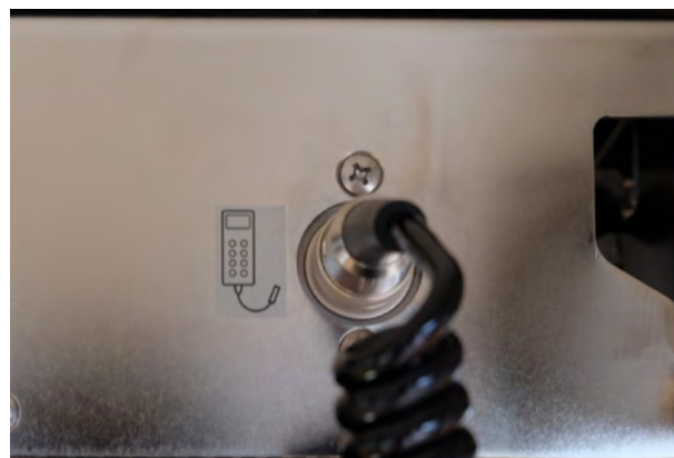
Fig. 4: Connection for the manual switch
