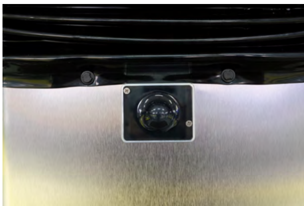
Fig. 3: Infrared receiver on the lifting column
