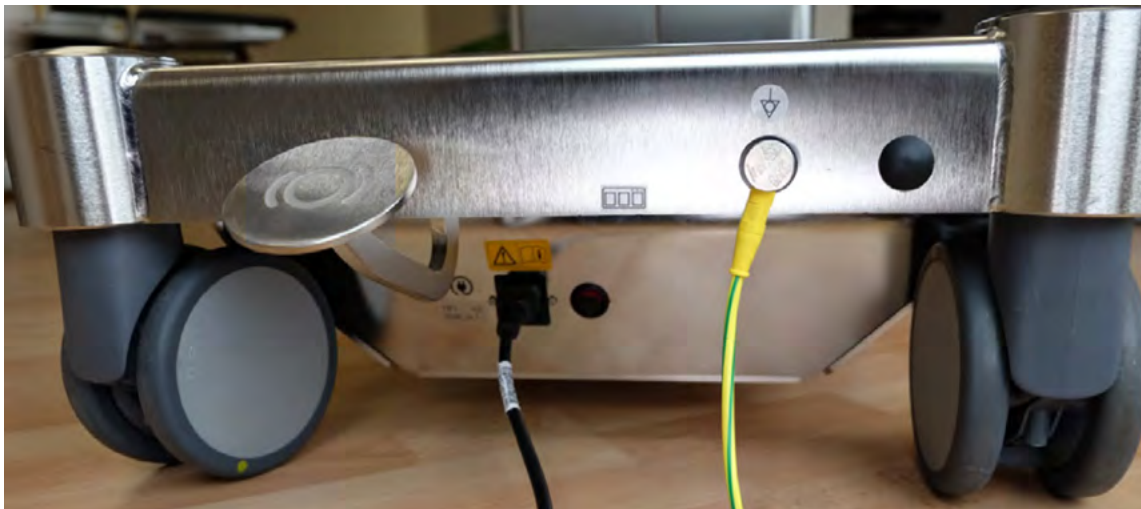
Fig. 5: Main switch and connections on the socket
